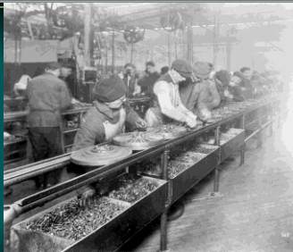
Assembly line for putting magnets on Model T flywheels, 1913
